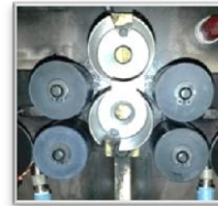
Arch wire under flex bending
